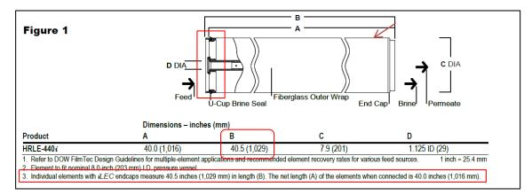
If we bear in mind that in the point 3 of the previous figure its indicated that, once all the elements are interconnected, each membrane fits in its following of the added measure 0,5" which this membrane have, the last membrane would sum up the total length of 40,5".
