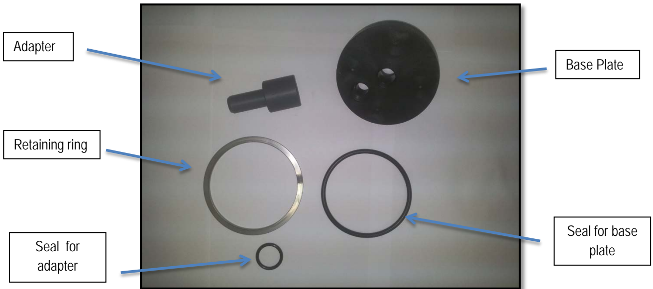
Fig 4.1 - Componentes cabezal BEL 4" - 300/450 psi Endport
